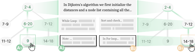
Fig. 5. Users can achieve quick assembling nodes by selecting any node in the tree graph as the tail of the chain. For example, after user clicks on node (A1) in outline view, the content in tutorial view (A2) updates correspondingly. (B1) and (B2) is another example.
