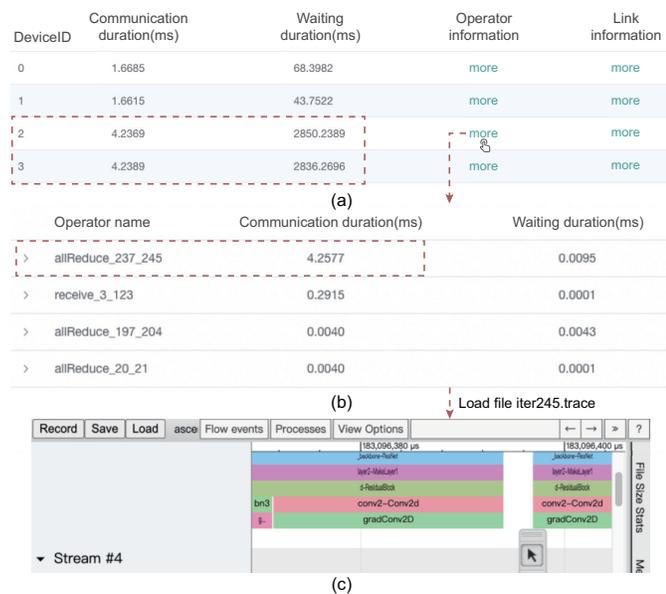
Fig. 14. The interactive analytic process using the Cloud TPU.
